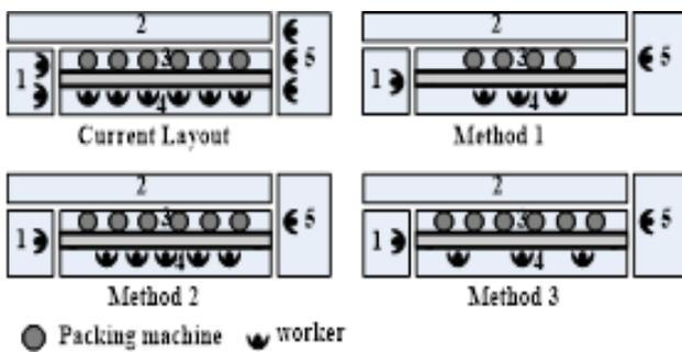
Figure 3. Comparison of layout of current and proposed methods
